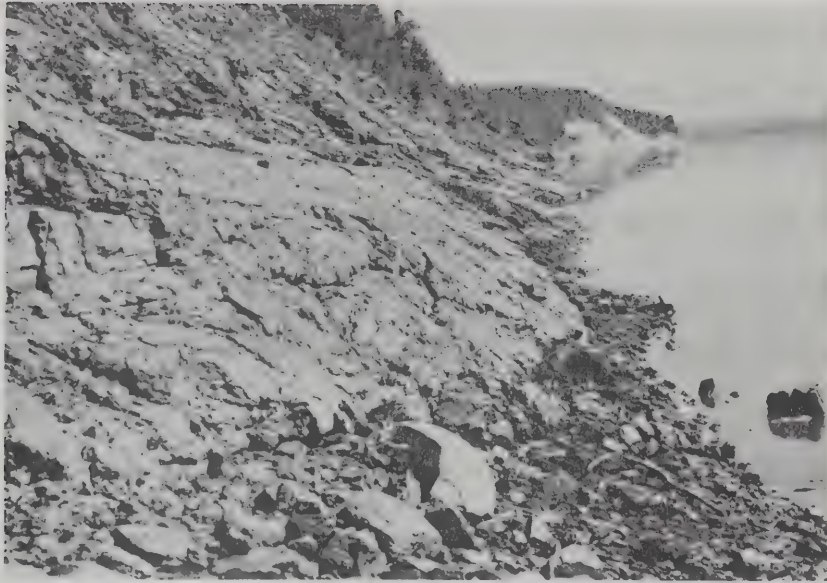
PLATE 3.5a Viscous Flow in Remoulded Oil Sand. The remoulded talus in the centre of the photograph has formed a viscously flowing 15° toe. Close examination shows other flows in the background.
